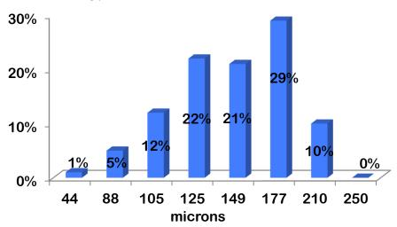
Average Particle Size: 163 microns Typical Bulk Density: 1051 g/L
